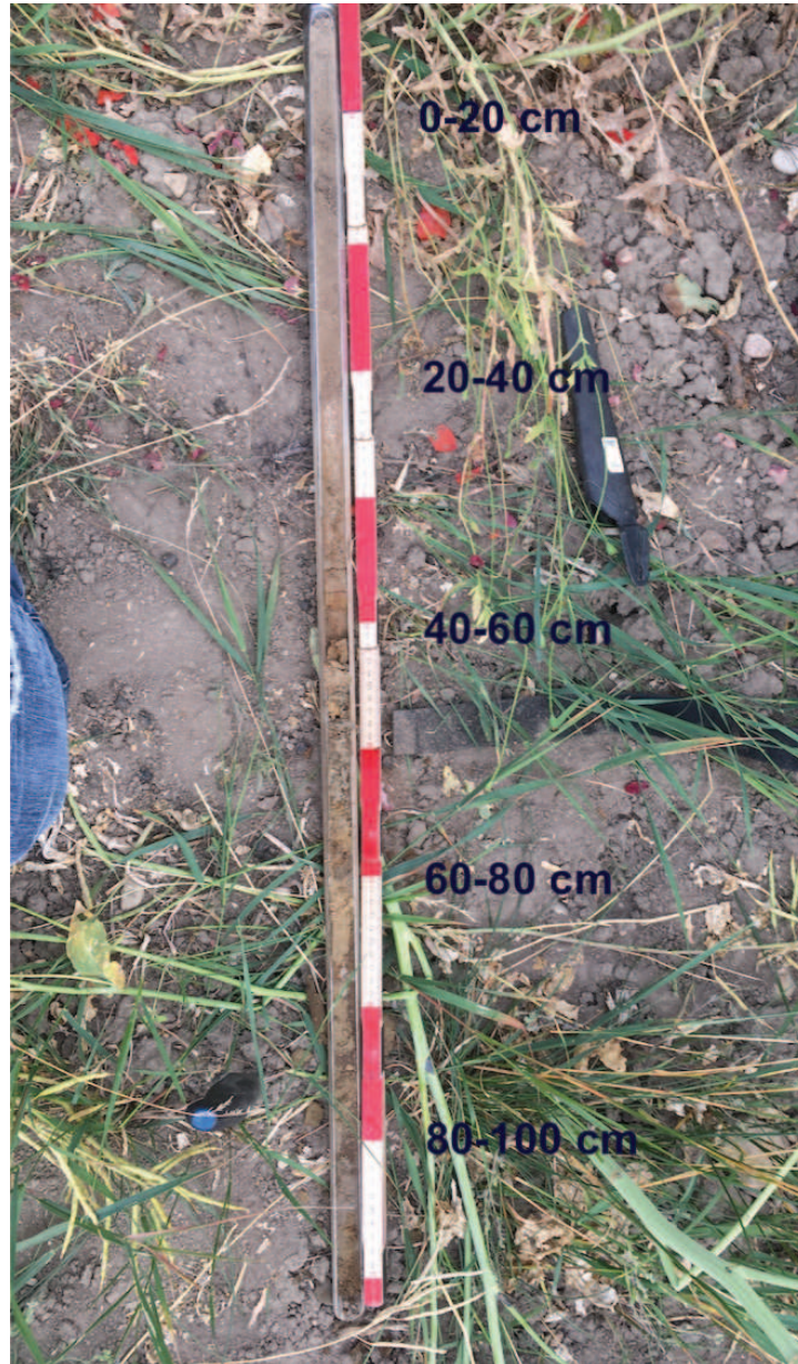
Figure 3: Soil auger with taken soil core. Schematic design of horizontal subdivision of depths.
