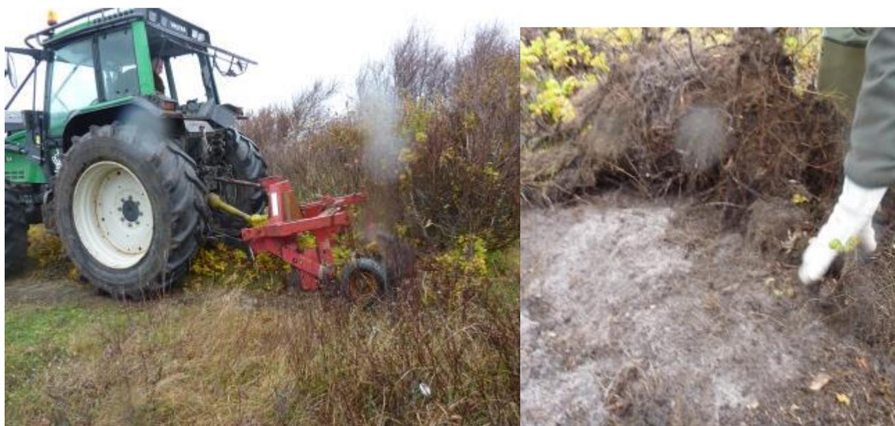
*The plant extirpator cut the rose bush free, lifts it and shakes sand and soil off the roots. (Photos R. M. Buttenschøn)*
