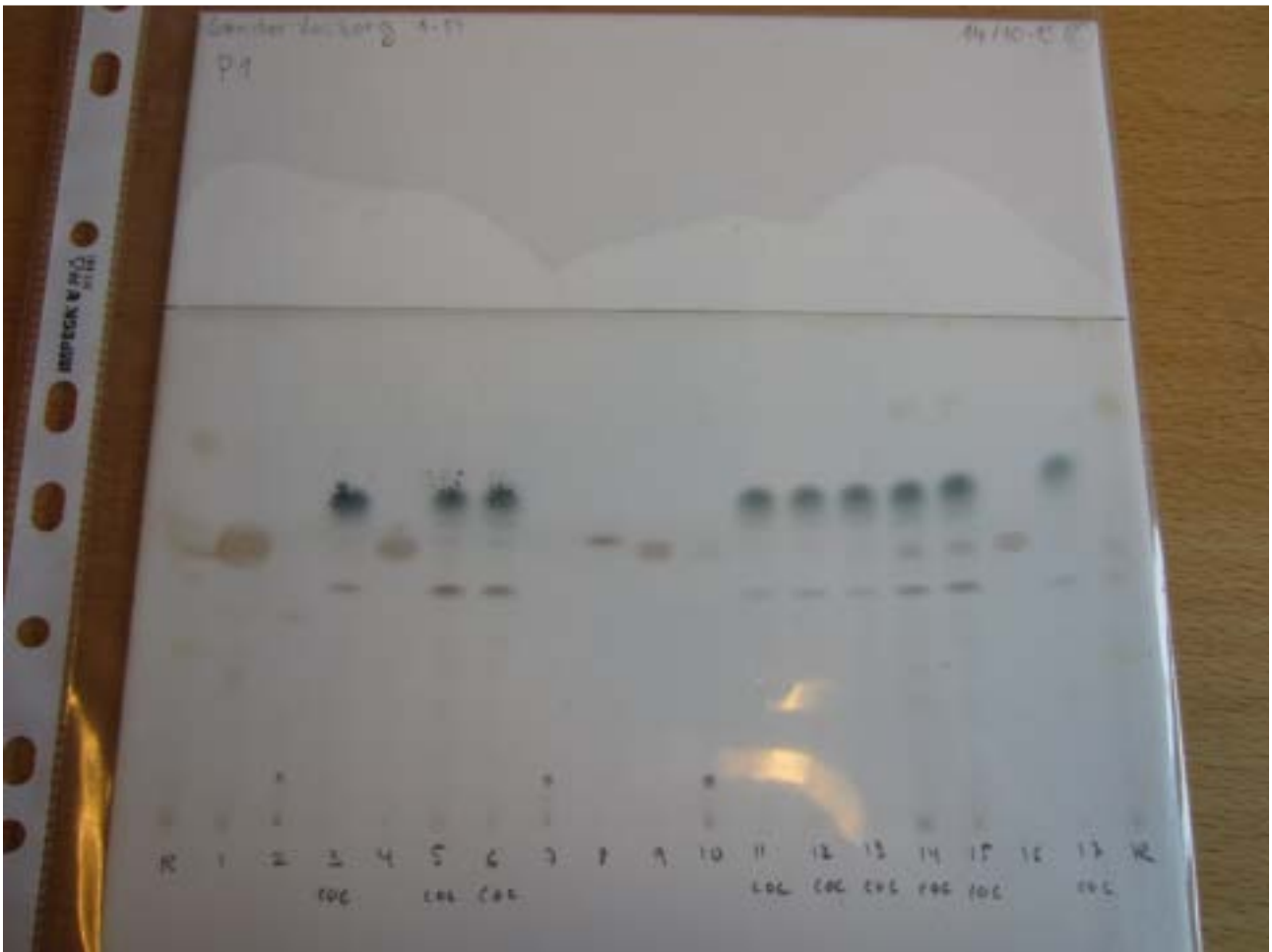
Picture 4. TLC plate from Sønder Vosborg Hede showing the problems experienced with the solvent.
