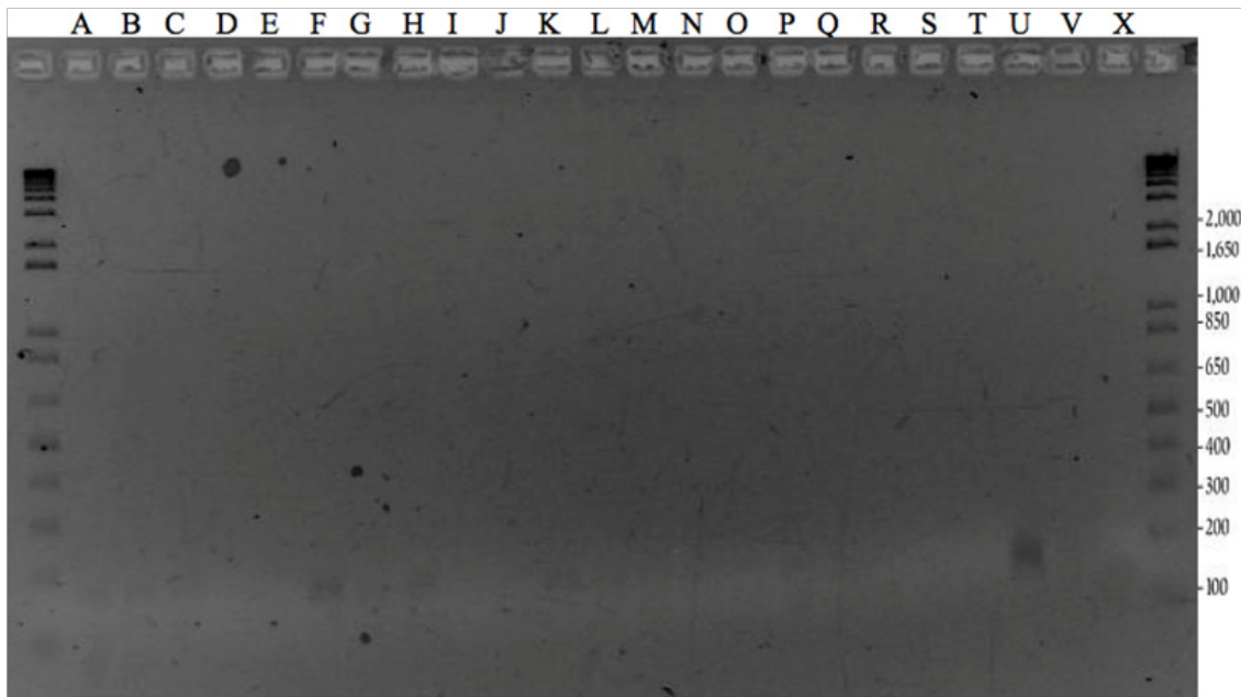
Figure 12. A representatives for the month August-December was loaded in order in dilutions 1:1 (A-E), 1:2 (F-J), 1:5 (K-O), 1:10 (P-T), Positive control (U) and negative control (V). All samples were run 40 cycles. 1-kB ladder available in both ends of the gel.
